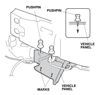
22. While wearing eye protection, drill the two pierced marks with a 3 mm drill bit, then enlarge the holes with a 5 mm drill bit. Remove any burrs. Do not damage the vehicle tube.
