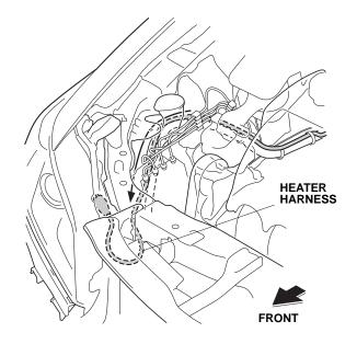
16. Using four black wire ties, secure the heater harness to the vehicle harness.
