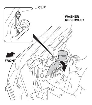
15. Route the heater harness toward the front of the vehicle and behind the washer reservoir. Continue routing the harness through the front bulkhead, and down into the bumper area.
