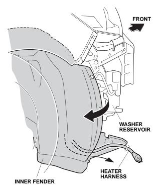
18. Using two black wire ties, secure the heater harness to the vehicle harness as shown.
