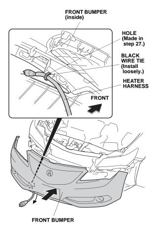
29. Tighten the black wire tie installed in step 28.
