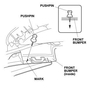
27. While wearing eye protection, drill the pierced mark with a 3 mm drill bit, then enlarge the hole with a 5 mm drill bit. Remove any burrs. To prevent drilling through the outer panel, wrap tape around the drill bit 10 mm (0.4 in.) away from the tip, or use a drill stop.
