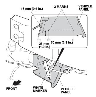
21. Using a pushpin, pierce the two marks on the vehicle panel.
