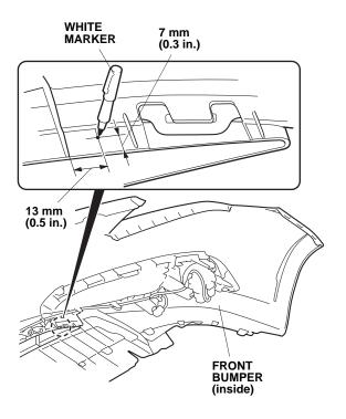
26. Using a pushpin, pierce the mark on the front bumper.
