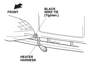
30. Attach the protective cap to the front bumper. Plug the heater harness connector into the protective cap.
