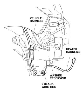
19. Using one black wire tie, secure the heater harness to the vehicle harness.
