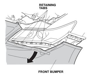
With the help of an assistant, remove the front bumper (unplug the vehicle connector, then release five pins and two hooks). Place the front bumper on a blanket to prevent damage.
