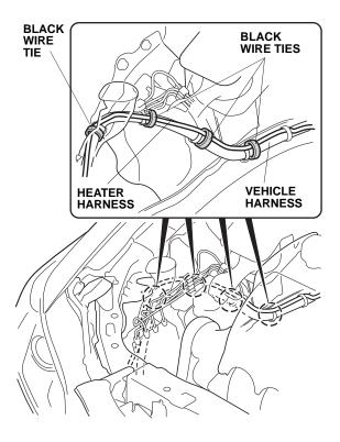
17. Pull the inner fender away from the washer reservoir, then route the heater harness as shown.
