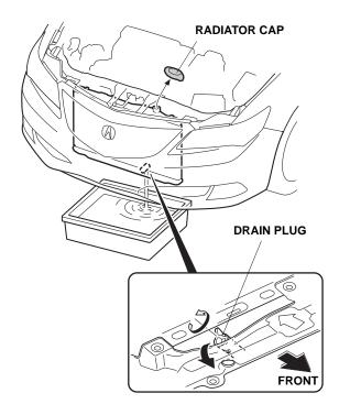
5. Drain the coolant completely, then replace the radiator cap.
