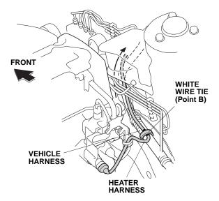
14. Remove the clip, then move the washer reservoir out of the way.
