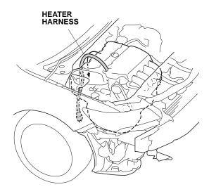
Remove the drain bolt. Coolant remaining in the engine jackets flows out of the hole when the bolt is removed. Retain the bolt; it will be used if the block heater is removed.
