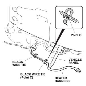
24. Secure the heater harness to the vehicle panel hole with one black wire tie as shown.
