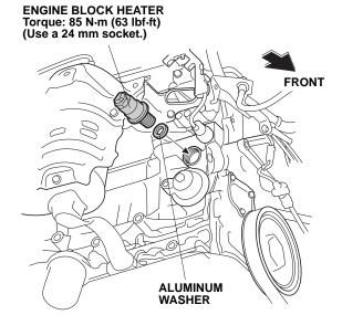
Plug the heater harness connector into the engine block heater. Make sure the heater harness connector is fully seated.
