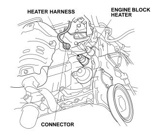
12. Secure the heater harness to the vehicle bracket with one white wire tie at the white mark (point A).
